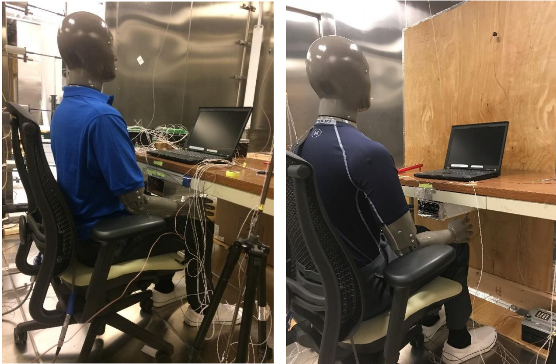
Figure 6-12 Manikin dressed in a polo shirt (left) and a sports shirt (right)
